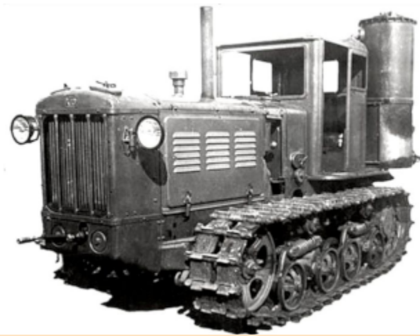
The KhTZ-2TG tractor, the wood-gas version of the SKhTZ-NATI tractor
