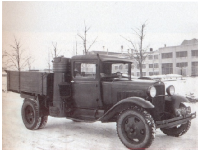
GAZ-43, a gas-generator vehicle that used anthracite to make coal gas 195
