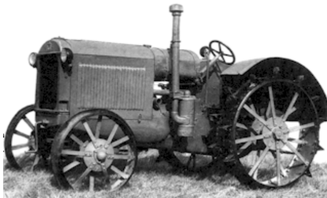
STZ 15/30 (aka STZ-1) agricultural tractor with a kerosene engine
